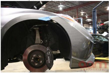
14) Remove 10mm bolts securing the bottom of bumper
