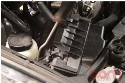
6) Remove PCV breather secured by a 10mm bolt, loosen clamp and completely remove PCV breather
