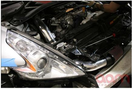
4. Replace existing radiator support bolt with supplied shorter allen bolt in order to clear lower intake pipe
