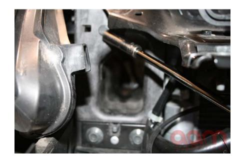
17) Using an air saw, router, grinder, dremel or any cutting tool. Open up intake air duct to fit new intake Before:
