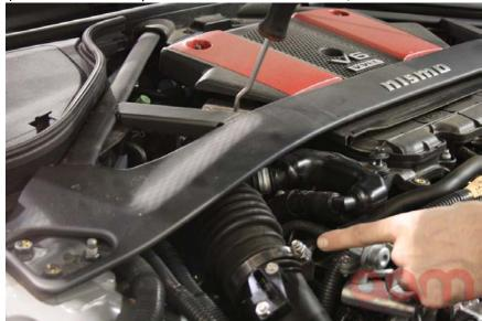
5) Remove 10mm bolt securing airbox
