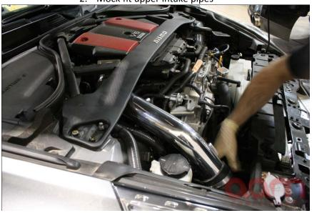
3. Mock fit lower intake pipes
