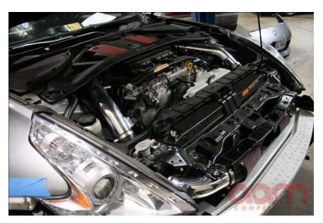
6. On the driver side, the PCV hose will clamp right onto the new intake
