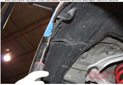
12) Remove 10mm screw securing bumper
